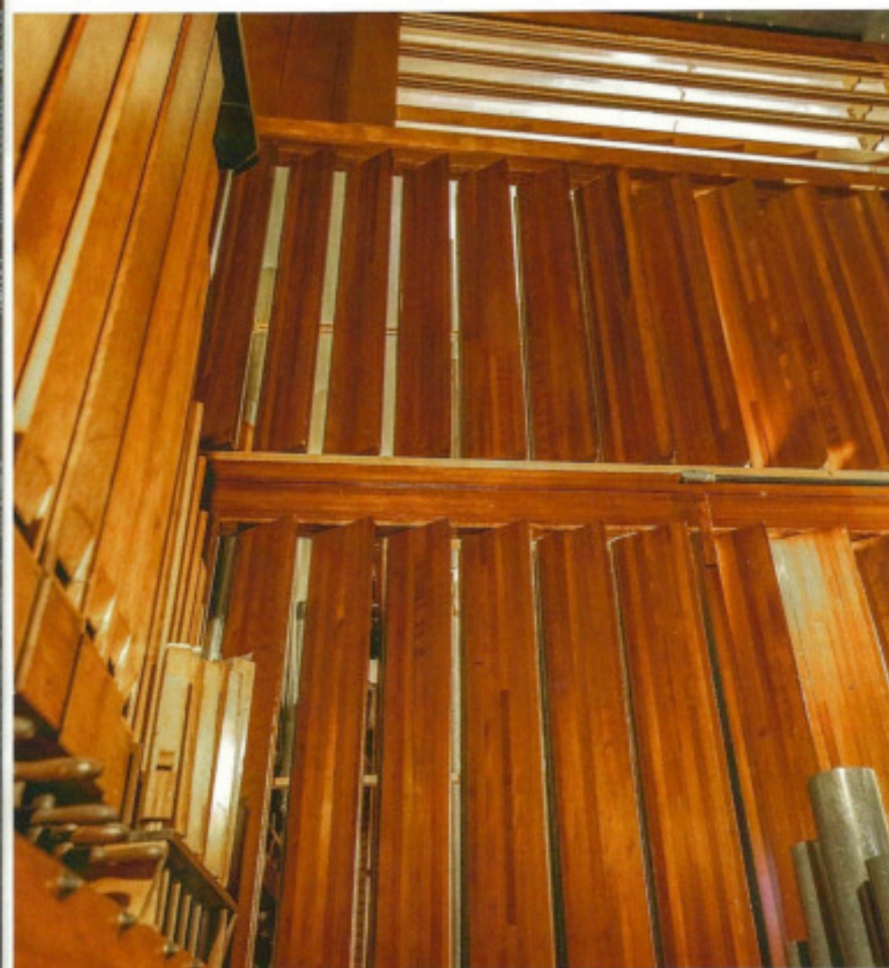
Inside the Woolsey Hall organ at Yale University, the 1915 Swell by Steere with vertical shutters, with added horizontal shutters by Skinner in 1928 to eliminate a tone pocket
